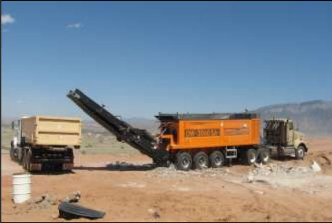
Figure 5. Doppsstadt® DW3060SA Crusher/Shredder
