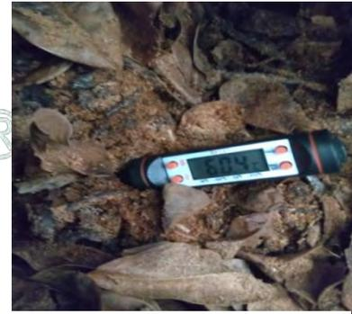
Figure 8 Temperature of an active pile recorded
