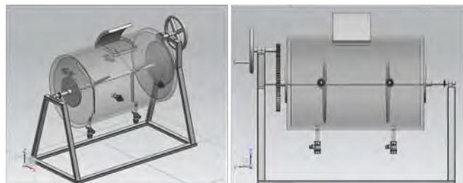
Figure 1. Schematic design of the Composting System (RGGC)
